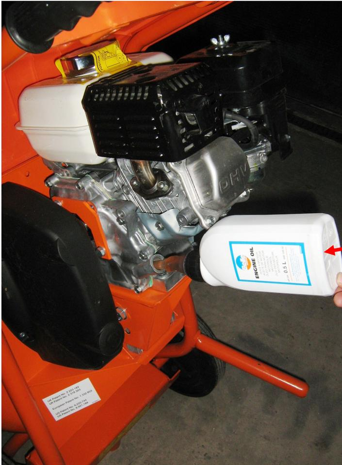
Fill the engine with the oil provided and ensure ALL the contents of the bottle are used.
