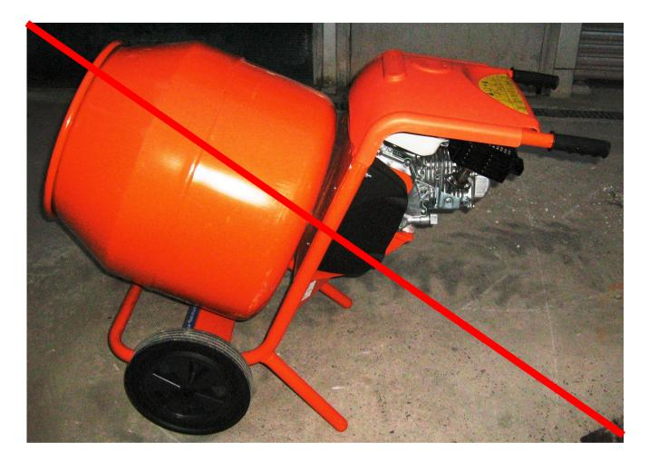
Do <u>NOT</u> check the oil in this position as this will allow oil to spill out, and then the oil alert will operate, and as a result the machine will not start.
