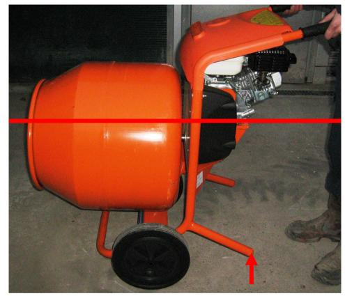
Machine checked in this position is correct, note person lifting mixer up so that engine is level to the eye.
