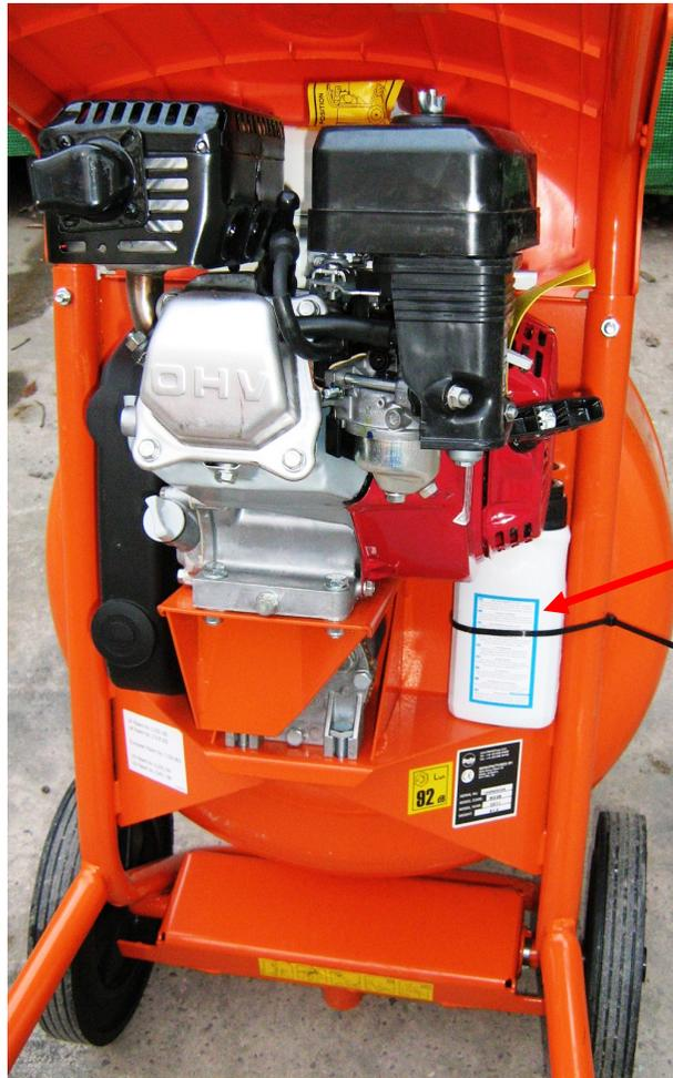
The machine comes with engine oil attached to the frame as shown.
