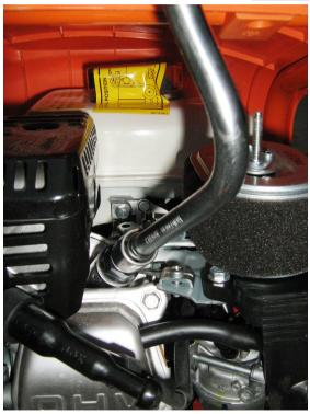
Using suitable plug socket and speed brace, or similar, carefully remove the spark plug,
