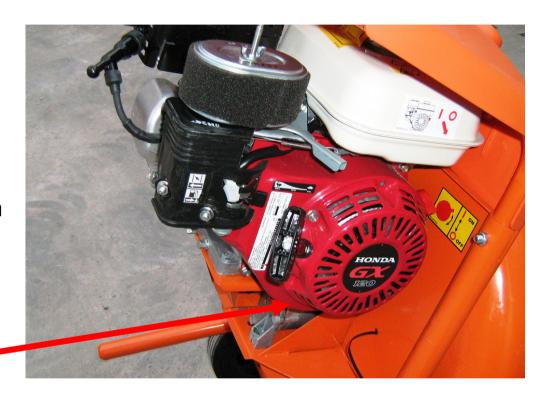
This Could be due to oil in the cylinder which in turn will cause hydraulic lock, which gives the impression of a seized engine.
