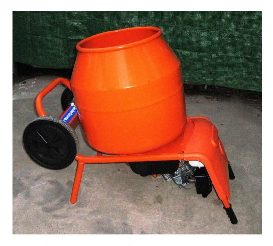
**Do NOT** transport mixer this way, otherwise oil will run into carburettor and also to the top of the piston.
