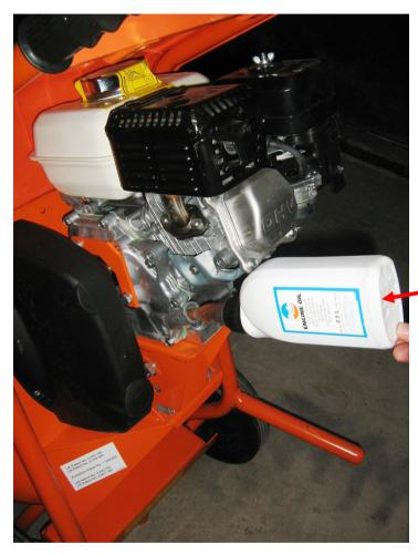
Fill the engine with the oil provided and ensure <u>ALL</u> the contents of the bottle are used.
